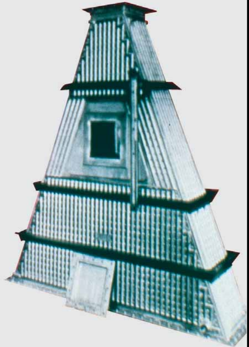
Water-cooled chute for a chemical product
