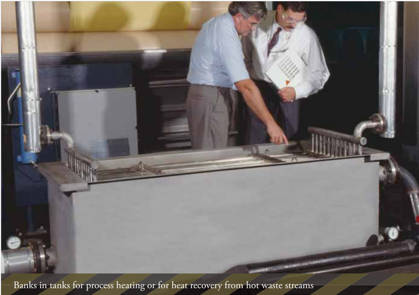
Curved alloy bank assembly for use in an agitated vessel
