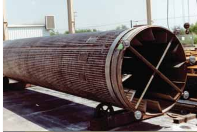
Bulk material dryer with heated baffles, commonly used in textile manufacturing and tobacco drying
