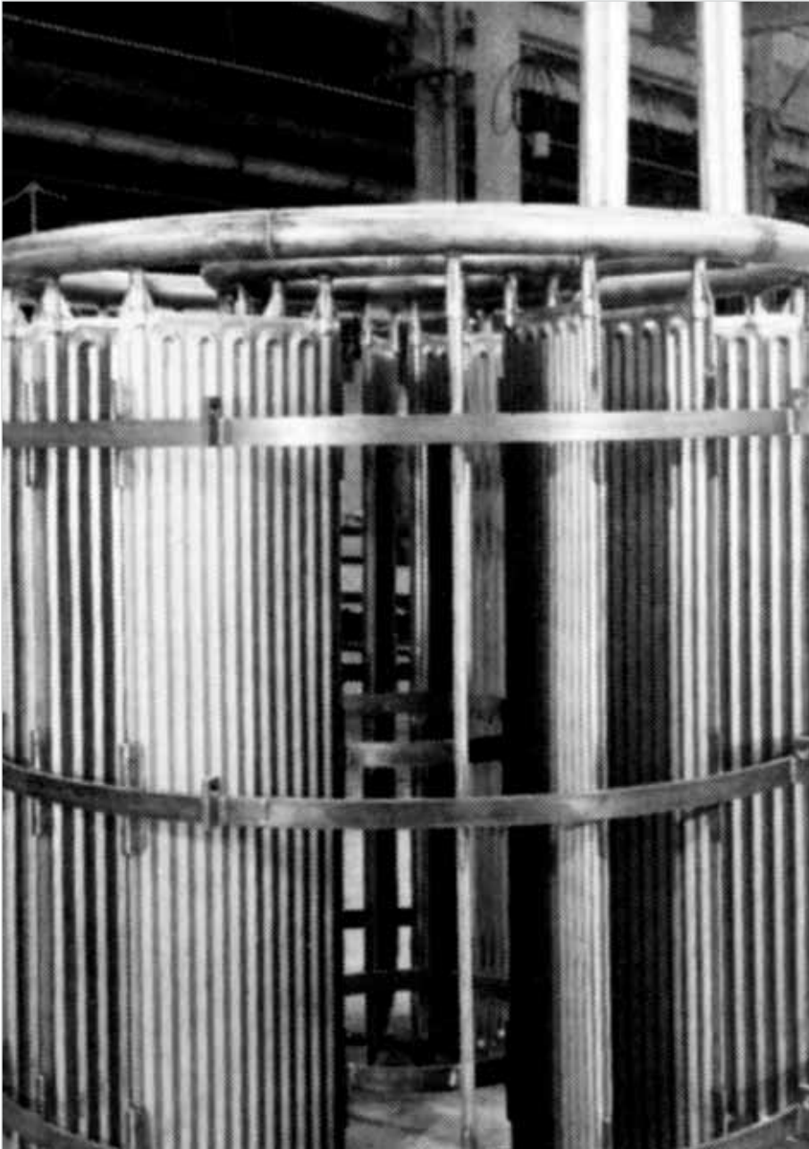
Circulator bank for use in a mildly agitated vessel
