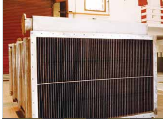
Waste heat recovery bank
