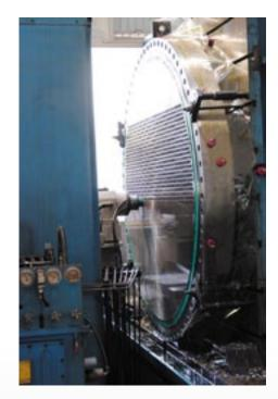
Maarky provides high, intermediate and low pressure feedwater heaters to the power industry for steam turbine applications ranging from 10 MW to 1,000 MW. The heaters can be designed for a variety of configurations including, but not limited to,:
